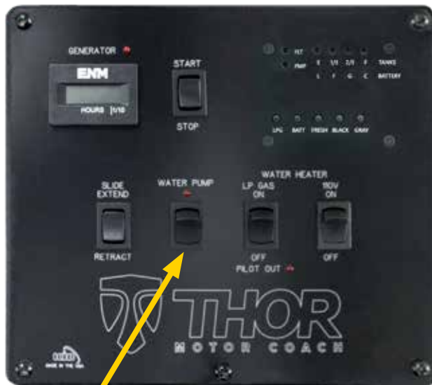
Water Pump Switch located on a typical Monitor Panel. The LED indicates power to the water pump.
