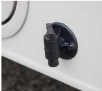
Typical fresh water tank drain valve
