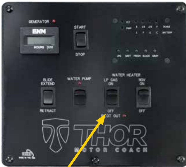
Water heater switch located on a typical Monitor Panel. Some water heaters are gas-only, while other models may feature both gas and electric heating modes.
