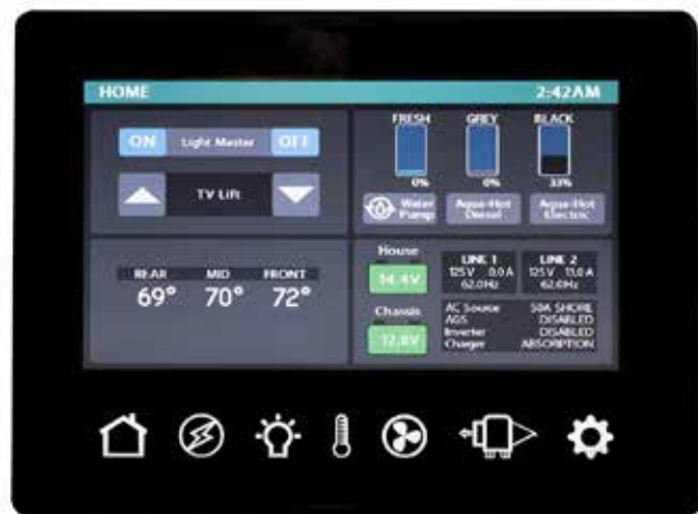
Typical multiplex main control panel. Electrical system monitoring is usually located on the main menu (house-shaped icon) screen.
