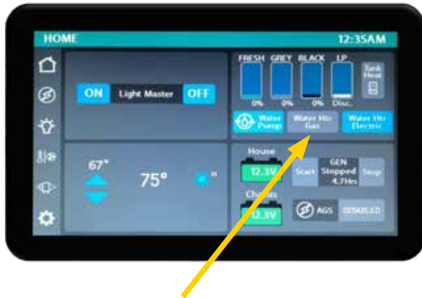
Water heater switch on a typical Multiplex control panel. Usually located on the Home Menu Screen, press the soft control to turn ON the water heater, selecting either gas or electric heating modes.
