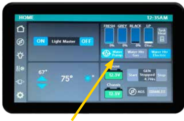
Water Pump switch on a typical Multiplex control panel. Usually located on the Home Menu Screen, press the soft control to turn ON the water pump. Press again to turn OFF the water pump.
