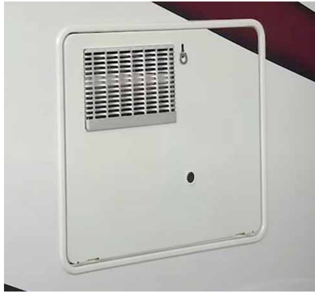
Exterior cover of a typical RV water heater. Peep hole in the cover is used to check for pilot light ignition.
