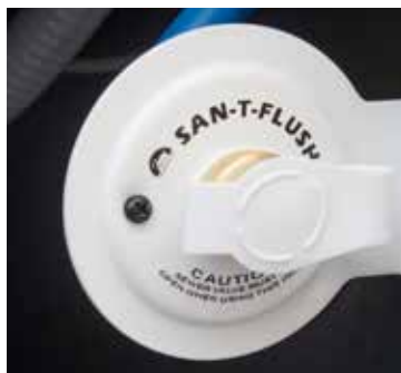
Typical black tank flush
