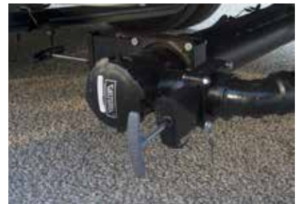
Typical Class C termination valve layout
