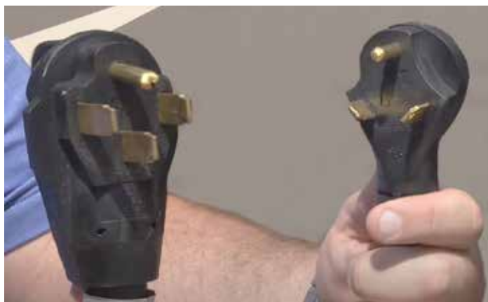
4-prong, 50 amp shore power cord (left) and 3-prong, 30 amp shore power cord (right)
