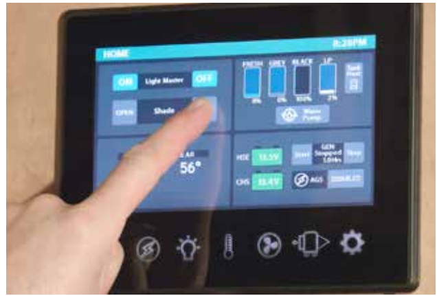
Multiplex switch panel illustrating the LP tank monitoring feature (upper right corner of the display area)
