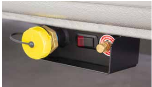
Propane access panel, positioned along the lower left side of the vehicle
