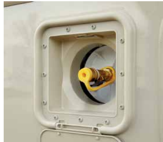
Typical external propane hook-up with quick-disconnect coupler
