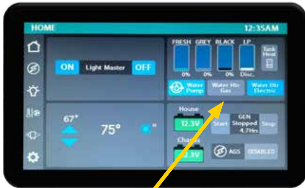
Water heater switch on a typical Multiplex control panel. Usually located on the Home Menu Screen, press the soft control to turn ON the water heater, selecting either gas or electric heating modes.
