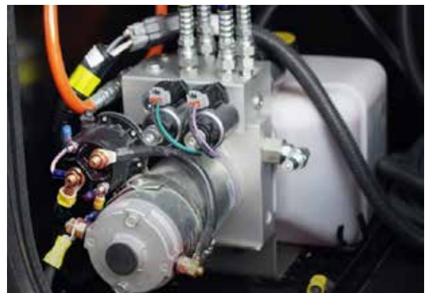
Typical Leveling Control Panels (above), which may contain an LCD read-out. Hydraulic pump assembly (below)
