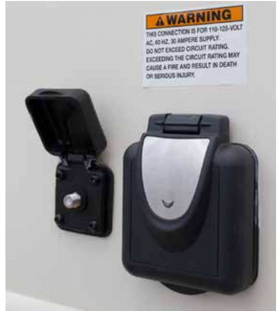
Typical park-supplied cable TV hook-up located on the driver's side of the motorhome. On some motorhome models, cable coax hookups are located on the fresh water panel.
