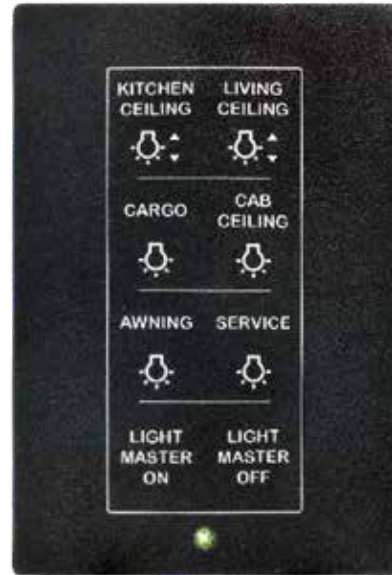
Typical multiplex wireless switch panel. Battery compartment access (below).
