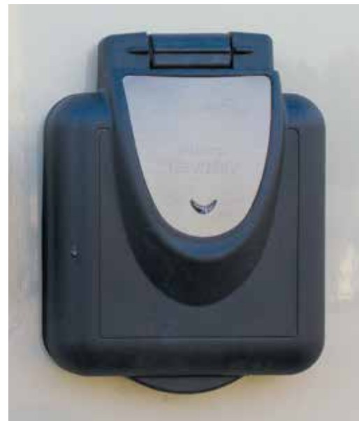
Typical shore line power port. Some power ports include a LED indicator that illuminates when power is ON to the motorhome.
