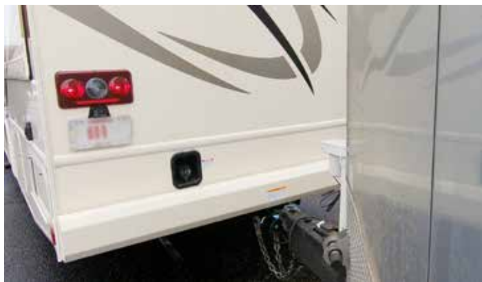
Towing a trailer with a standard trailer coupler
