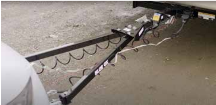
Flat towing with a tow bar
