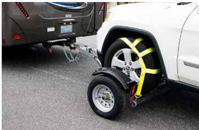
Towing a vehicle with a tow dolly
