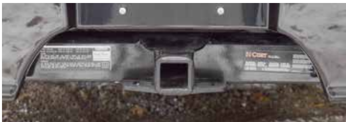
Hitch ratings are printed on labels affixed to the tow hitch
