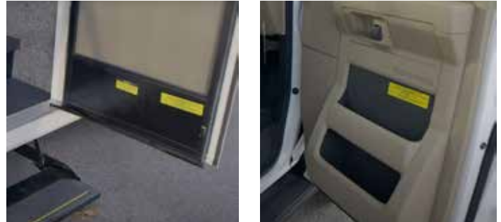
OCCC Label is affixed to the most forward right-side entry door of the motorhome (Left: Class A, Right: Class C).
