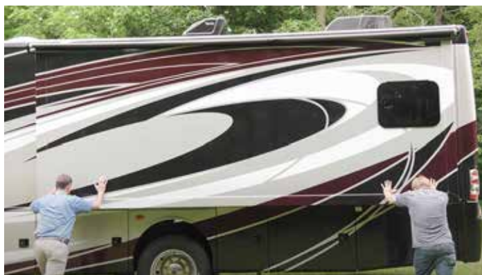
Figure 5: Pushing in a slideout
